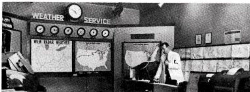
Crosley's fully equipped weather center, with Tony Sands, chief meteorologist. Equipment includes the weather radarscope and the six basic instruments for recording temperature, wind pressure, humidity and rainfall and transmission equipment for weather maps and weather bureau messages.
